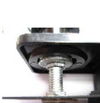
Nuts/washers installed between L bracket and faceplate
