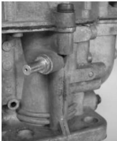
*4-mm hole, and cutting M5-thread into the dual choke carburettor (see photo) because these are already prepared for a vacuum nipple. The nipple is supplied with the 123\|EVO.*
